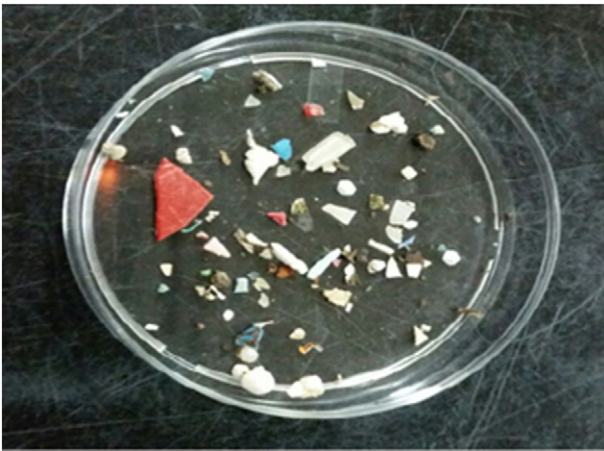
Fig. 2. Microplastics in different sizes and color from mangrove sediments in Peninsular Malaysia.
